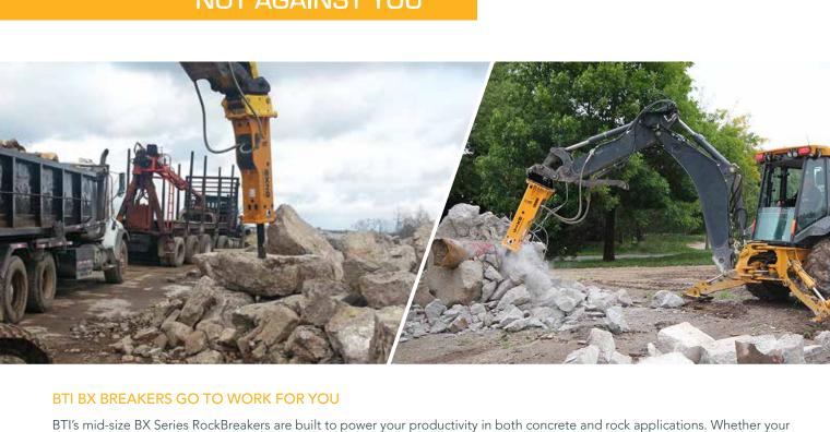
BTI's mid-size BX Series RockBreakers are built to power your productivity in both concrete and rock applications. Whether your job is breaking down concrete surfaces, trenching, or preventing blockage in crushing systems, our BX Series RockBreakers are made to withstand continuous breaking in harsh environments.
