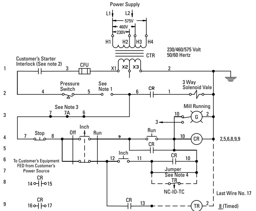
Normal mill starting procedure is to bring the motor up to operating speed and then engage the clutch to accelerate the mill. Airflex offers a simple, but very reliable system for clutch control. The system consists of two parts: the pneumatic and electrical portions.
